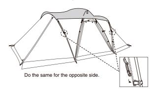
⑥Attach the remaining eight hooks on the roof sheet to the rings of the tapes with plastic hooks on the main unit.
