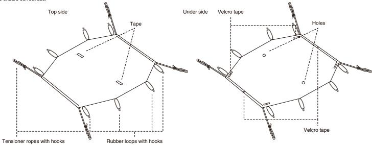
①Spread the roof sheet with the bottom side (side with velcro tapes and holes) i ②With the roof sheet upside-down, wind the two velcro tapes on the main unit facing up, in front of the shelter.
